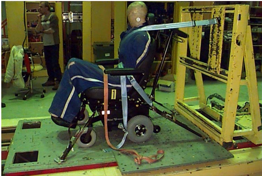
Belt system before test.
